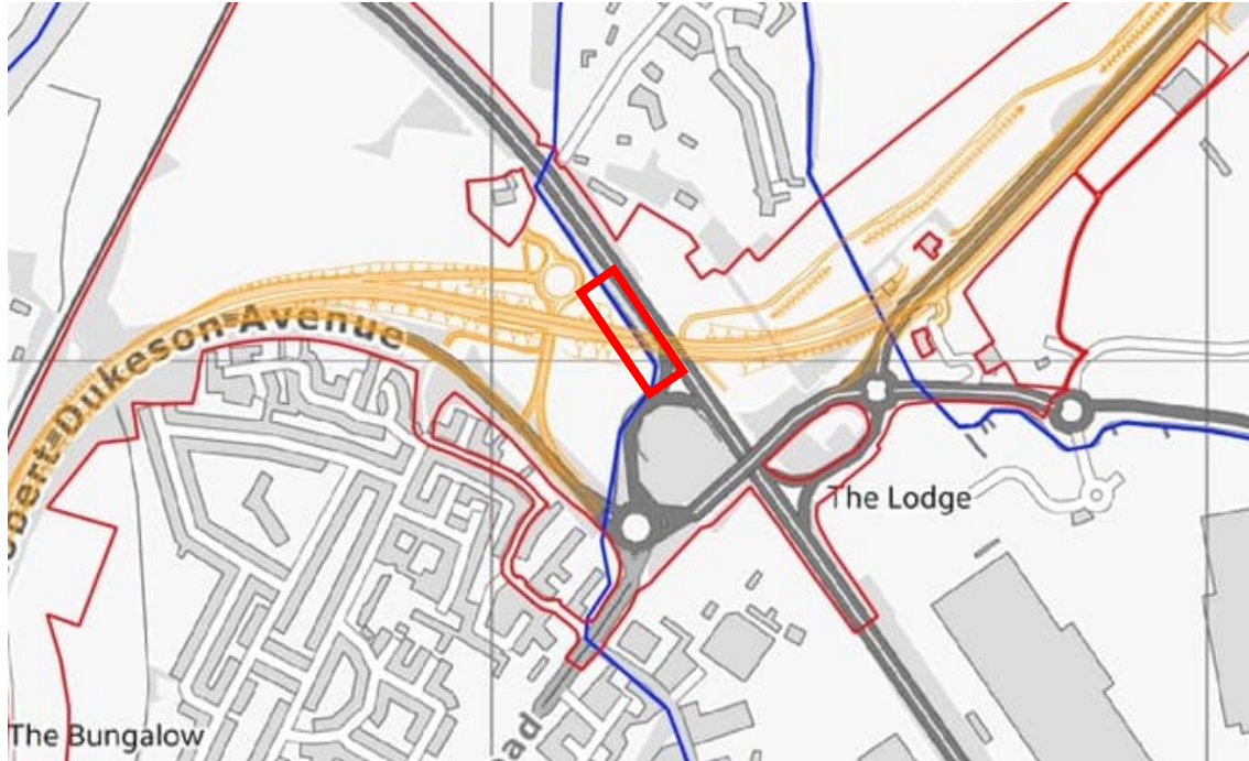
Figure 3-2: Realigned Slough Dyke in relation to Scheme alignment, with the realignment area highlighted in red
